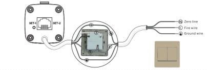
AC power switch double button mode four-wire connection method:
